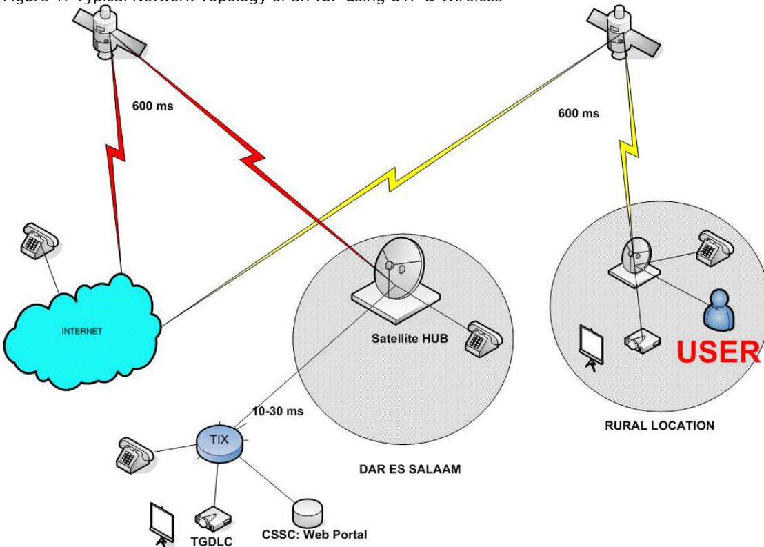
Figure 2: Standard Topology of a Satellite provider having an International Satellite Hub
