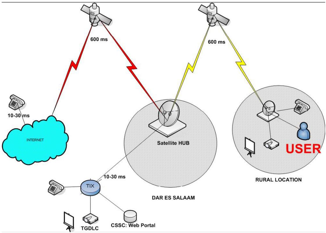
Figure 3: Standard Topology of a Satellite provider having a Local Satellite Hub
