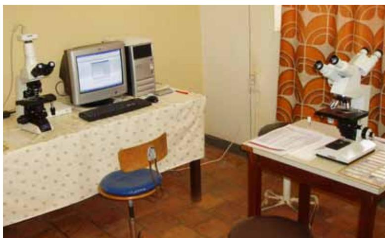
The camera connected to the left microscope is used to digitise tissue samples and send them to specialists.
